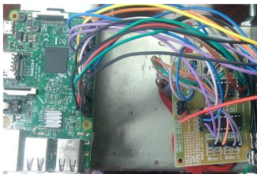
Figure2: Circuit connection of Raspberry Pi and L293D Figure3: Circuit Connection of Ultrasonic Sensor
